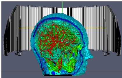
Figure 1: The head model (blue) with the blood vessels (red), and a part of the coil (grey).
