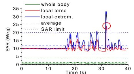
Fig. 3: Global and local SAR changes due to different movements inside the scanner. Up to 240% SAR increase was observed in this example.
