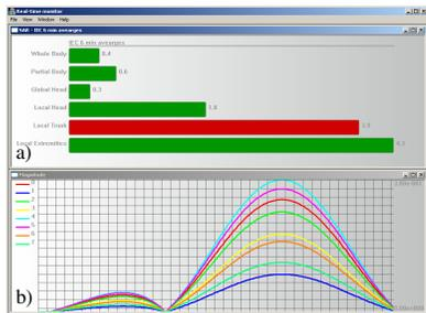
Fig. 1: Real-time display of global/local SAR with SAR violation in red (a) as well as the RF pulses for each RF Tx channel (b).
