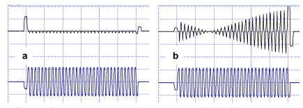
**Figure 1.** Transverse gradients used for a conventional EPI 2D RF pulse excitation (left) and the same sequence modified to enable acquisition of an image during the flyback of the EPI pulse sequence, in between RF pulses. The blipped gradient is not set to the same scale in the two figures. The sequence allows k-space to be traveled along the optimal line needed to compensate for the RF coil phase during each flyback, and then return to the proper position for the RF pulse generation.
