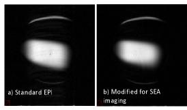
Figure 3. (left) Images of a circular phantom with an inner volume selected using a 2D RF pulse from standard blipped EPI approace (Fig 1a) and with a pulse sequence modified to enable SEA imaging during the flyback period (Fig 1b).
