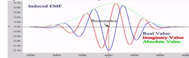
Fig.5 A shielded coil, with a sample introduced resonance at \approx 400 MHZ
