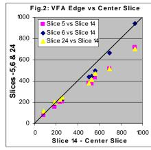
IR-FSE shows good agreement at all locations (Figure 1), one can observe significant deviations at the edge slices with 3D VFA.
