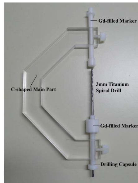
Fig.1 Custom-made navigation device with opposite markers for visualization
