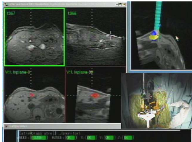
Fig. 2 A display of our navigation software. The upper left 2 windows are real-time MR images in 2 perpendicular planes and lower left 2 windows are reformatted images from 3D data in the corresponding planes. The tumor area is shown in red. In the 3D display (upper right), tumor volume is shown in yellow and the treated volume is shown in blue.
