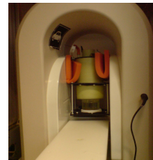
Figure 1d. Phantom imaging setup in Niche MRI scanner
