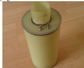
Figure 1c. Cryogenic Dewar, made from G10 materials
