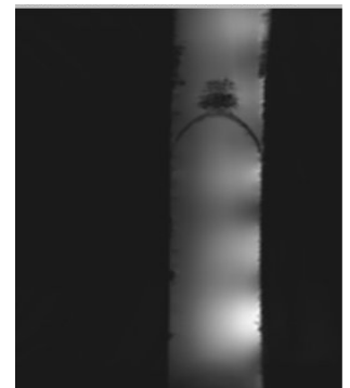
Fig.3 The 7T MR imaging result of a water phantom with structures.
