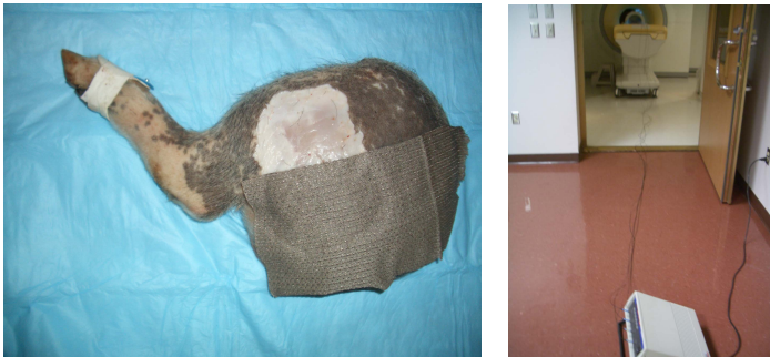
Figure 1 a) Placement of the silver containing wound dressing on a porcine skin wound. b) Experimental setup of the Luxtron 790 Fluoroptic Thermometer and the fiberoptic cables in the 7T.
