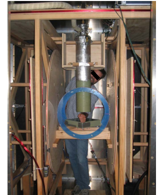
Figure 1: Photograph of the SQUID-MRI system configured for in vivo imaging of the forearm.
