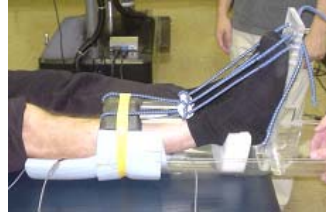
Fig. 1. MRI-compatible cradle for leg immobilization with adjustable ankle joint positions.
