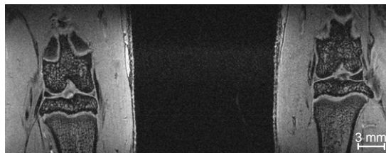
Fig. 2: Image acquired simultaneously using two similar two-channel array coils positioned on the right and left rat knees.
