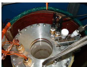
Fig.2 Top flange contains the required feedthroughs, including the polarizing cell gas line for adding and removing hyperpolarized helium.
