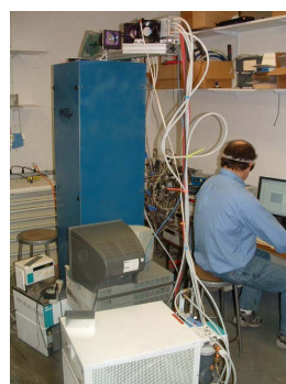
Fig.3 First assembled system shows the high power laser temporarily mounted on top of the vertical metal box containing the polarizer.
