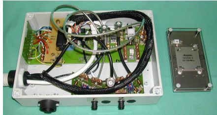
Fig. 1 Interior of T-R switch built for ^3\text{He} at 97 MHz
