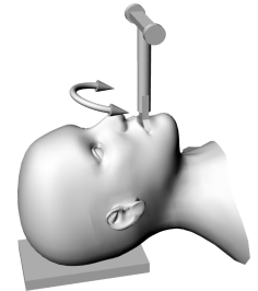
Fig. 1: Excitation device and resulting head motion (arrow) consisting of a combined nodding and left-to-right motion.
