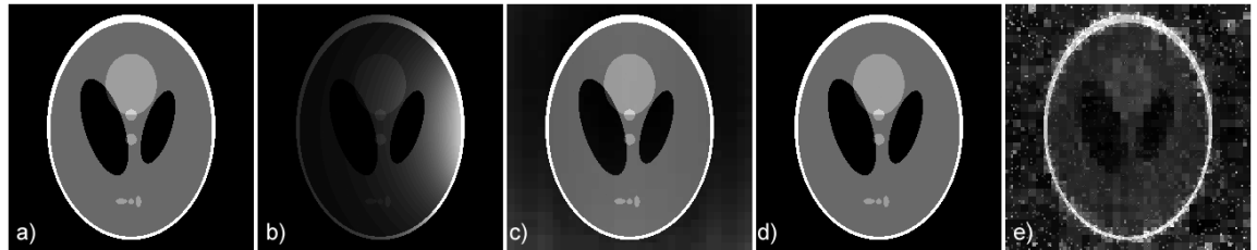
Figure 1: Shepp-Logan phantom, a) original, b) simulated ideal coil image, c) 4000 wavelet coefficient reconstruction by SOMP from 15,000 measurements, d) SOMP reconstruction with 10,000 measurements and e) SOMP reconstruction with 5,000 measurements showing degradation in agreement with theory.
