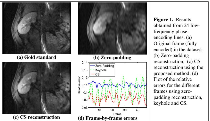
**Figure 1.** Results obtained from 24 low-frequency phase-encoding lines. (a) Original frame (fully encoded) in the dataset; (b) Zero-padding reconstruction; (c) CS reconstruction using the proposed method; (d) Plot of the relative errors for the different frames using zero-padding reconstruction, keyhole and CS.
