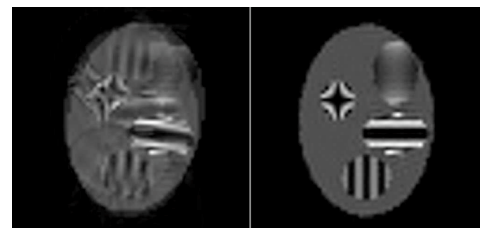
Figure 3: Images of the object reconstructed from motion-corrupted signals: with conventional GEM (left) and motion-corrected with the motion-adjusted GEM formulation (right).
