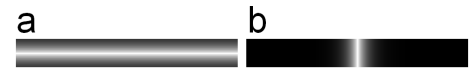
Fig.1 k -space weighting schemes for single blade of LAP-EPI (a) and SAP-EPI (b) at a \lambda of 0.1. Note that the phase encoding direction is vertical in a and horizontal in b.
