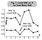
**METHODS.** We use FDTD methods at 300 MHz in a human head model [1] to derive the *E* & *B* fields for each coil at locations **r** per Amp. of current in an array of eight,  $15_{cm}$ -dia. overlapping loops spaced by  $45^{\circ}$  on a  $28_{cm}$ -dia. cylinder.  $B_1^+$ fields are formed and used in a Bloch equation simulator to model pTX excitations.
