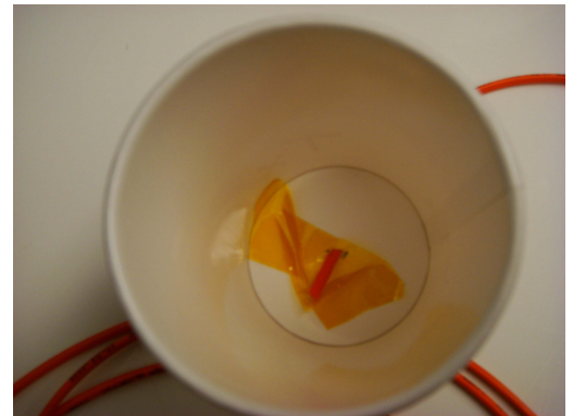
Figure 1: Depicting communication device construction, including audio transceivers and fiber optic transmission line, which is terminated at high performance polyimide tape bond.
