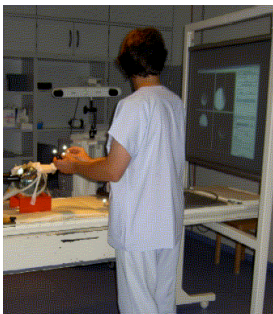
Fig. 1: Overview of the in-room components (see also Fig. 2): instrument tracker and holder, marker holder, tracking camera, and rollaway screen.
