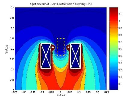
**Figure 2.** Normalized magnetic field profile for the shielded polarizing magnet (large rectangles). The white dots indicate shielding coil locations and the yellow rectangle indicates PMT location.
