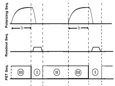
**Figure 3.** Pulse sequence for interleaved PET/FCMRI. Region I and II correspond to the time when MR and PET operate independently. Region III indicates where PET can operate simultaneously with FCMRI as a result of shielding the polarizing magnet. This increases the duty cycle of PET by a considerable amount.
