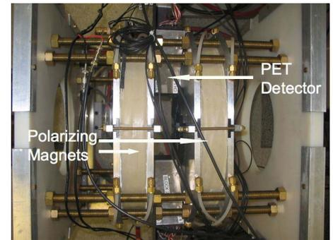
**Figure 1.** Polarizing magnet model with integrated PMT detectors.
