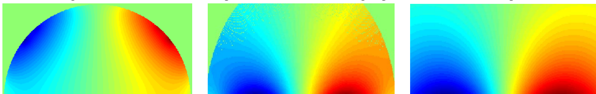
Figure 2. Simulated B-field map. (a) Field map from conventional cylindrical wire pattern, (b) Conformal mapped B-field map from (a), (c) B-field map from planar wire pattern, which is conformal mapped from same cylindrical wire pattern. Note that current distribution on the bottom for (b) and (c).
