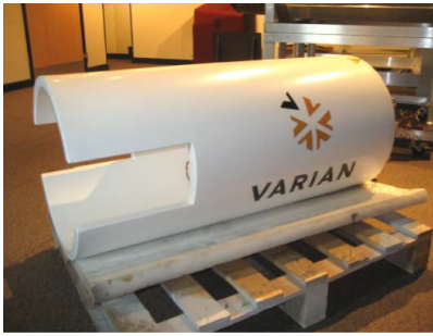
Figure 2. The completed gradient and shim coil set.
