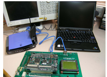
Fig2. DSP with DDS, ADC, controlled pre-processing circuit and Ethernet
