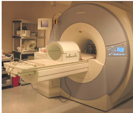
Figure 2: Photo of the 128 channel system with the 128 element lung array for hyperpolarized 3 He on the patient table
