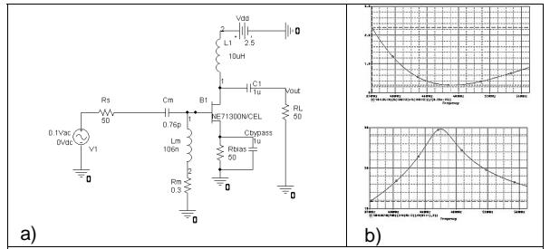
Fig 2. a) circuit with matching components, b) NF (top) and Gain plots at 470 MHz
