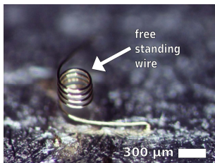
Fig. 2: Air coil after core removal.
