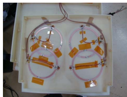
Fig.2 Layout of the coil elements inside the upper and the lower components
