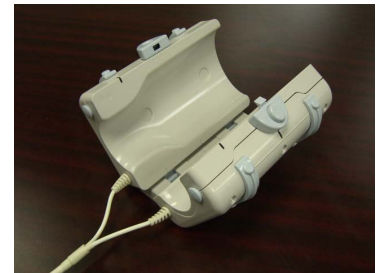
Fig. 6 Mechanical design of the wrist coil
