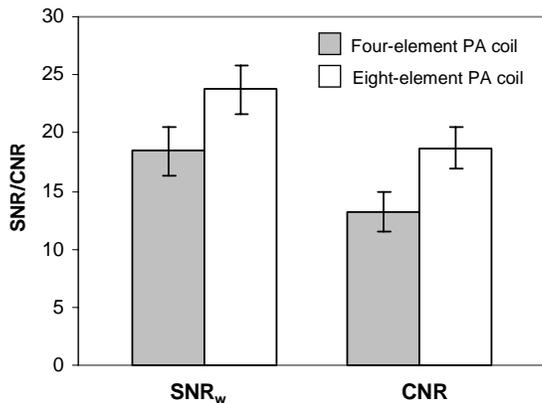
Figure 1: Improvement in SNR and CNR of eight-element PA coil over four-element PA coil on ultra-high resolution (0.27m in-plane) T1 images
