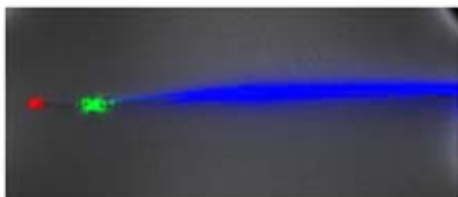
Fig 2. Catheter in water phantom with color overlay for each channel. Red corresponds to the loop coil at the distal tip, green to the loop coil 3 cm down, and blue to the monopole antenna.
