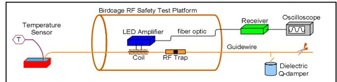
Figure 2 (left): Schematic of the optically-coupled system for measuring RF guidewire currents. Figure 3 (above): Setup on the birdcage RF safety test platform for measuring guidewire currents and validating the effectiveness of devices realized to reduce them.
