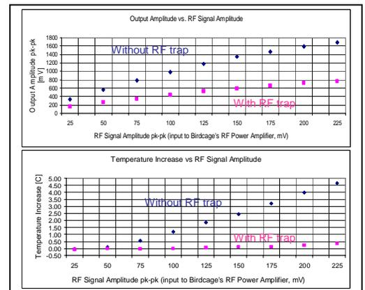
Figure 5 (above): Effects on the guidewire currents (top) and heating (bottom) by a RF trap, at several different values of the MRI RF signal
