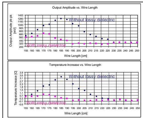
Figure 4 (above): Effects on the guidewire currents (top) and heating (bottom) by a lossy dielectric, at several different lengths of the wire
