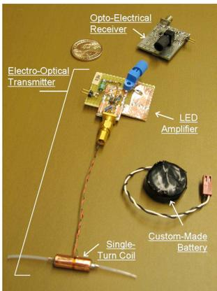
Figure 1 (above): Picture of system for measuring RF guidewire currents.
