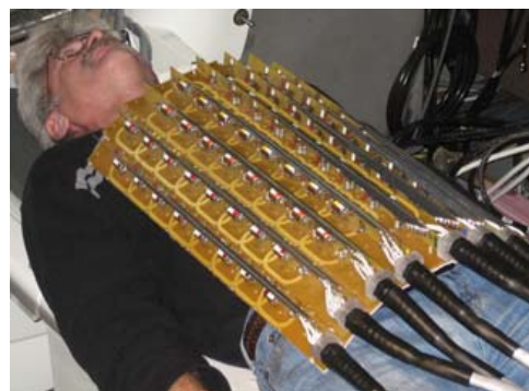
Figure 1. Flexible 64-element anterior RF coil array, with covers removed, on a subject lying on the 64-element posterior array.
