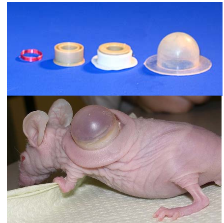
Fig 1: (top) RF coil, PEEK coil former, base ring and cap of a skin chamber. (bottom) skin chamber after implantation into a nude mouse.
