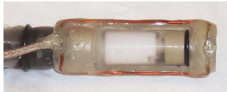
Figure 1. Head of the integrated endoscopic device (with the coil positioned outside the balloon).
