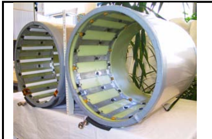
Fig.2: Two shielded coils were built, on the far left within a GRP supporting tube, on the right hand side within a sandwiched cylinder of 7,5 mm GRP and 7,5 mm foam
