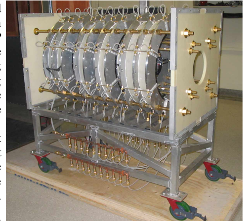
Figure 1: The field-cycled MRI scanner developed by the authors.
