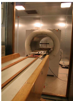
Fig 1. 15mT very low field MRI system.
