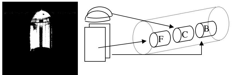
Figure 3 Axial and coronal GRE images acquired with a shielded Tx/Rx RF surface coil. These images were acquired with the surface coil on top of the water bottle while the grid phantom was in the opposite region. Left images are from the front region (correct gradient polarity), Right image pair is from the rear region (reversed polarity images). Window/Level chosen to illustrate lack of cross talk from opposite region.
