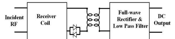
Figure 1: Generalized schematic of scavenger circuit attached to the receiver coil.
