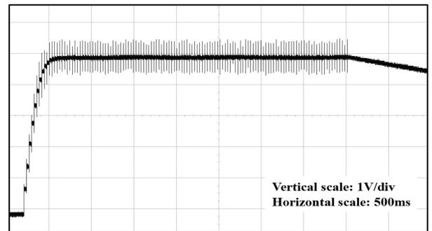
Figure 2: Scavenger output during a single 8.5s GRE acquisition (TR=30ms,  $\alpha=25^\circ$ ). The circuit is immediately charged and is sustained between RF pulses.
