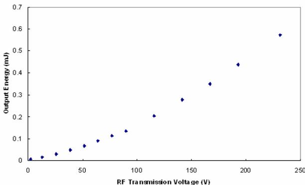
Figure 3: Energy stored in 10uF capacitor based on the amount of transmission voltage.
