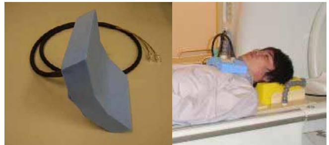
Fig. 2 2-channel receiver coil dedicated to esophageal imaging
