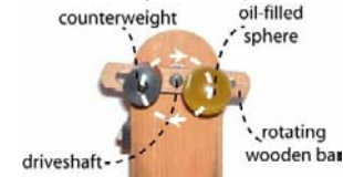
Figure 1: Picture of phantom. Dashed line represents path traced by sphere. Motor is connected to driveshaft.
