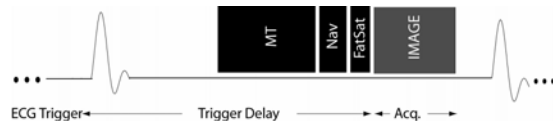
Figure 1: Coronary vein imaging sequence: a magnetization transfer (MT) preparation, consisting of 8-10 off-resonance RF pulses, is followed by respiratory navigator (NAV) and spectral selective RF for fat saturation (FatSat). A gradient echo or SSFP imaging acquisition composed of 10-15 imaging TRs is applied for image acquisition (IMAGE).
