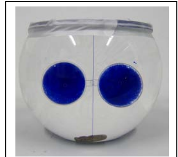
Figure 1: Phantom setup, hollow spheres containing differently generated capillary networks, a single string is mounted vertically, i.e. perpendicular to the main magnetic field.
