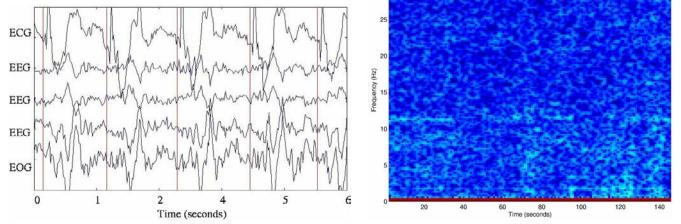
**Figures:** Left figure shows example signals before pulse artifact subtraction during the first few seconds of the scan (rest). Right figure shows a corresponding EEG spectrogram demonstrating alpha activity only in the resting periods, especially the first one ending after 30 seconds.
