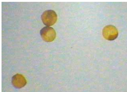
Figure 1. The ferrite-containing polystyrene micro-beads with the diameter of 20 \mu m.
