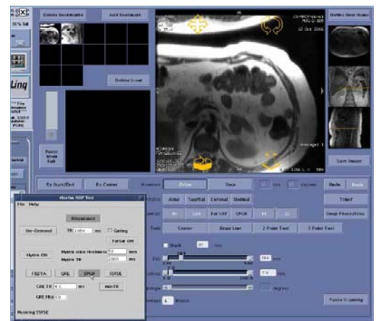
Fig. 2: The RTGS controller interfaced to i/Drive and running an SSFSE sequence axially in the mid- abdomen of a volunteer.
